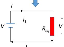
$$V = V_1 + V_2 = IR_1 + IR_2$$
