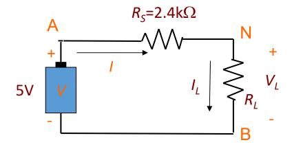
Can you plot the graph Power at  $R_L$  vs  $R_L$ ?
